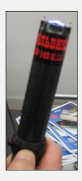
**◄** Electric shock baton with two electrodes
