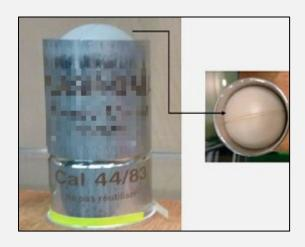
▲ 44 calibre cartridge with single rubber ball
