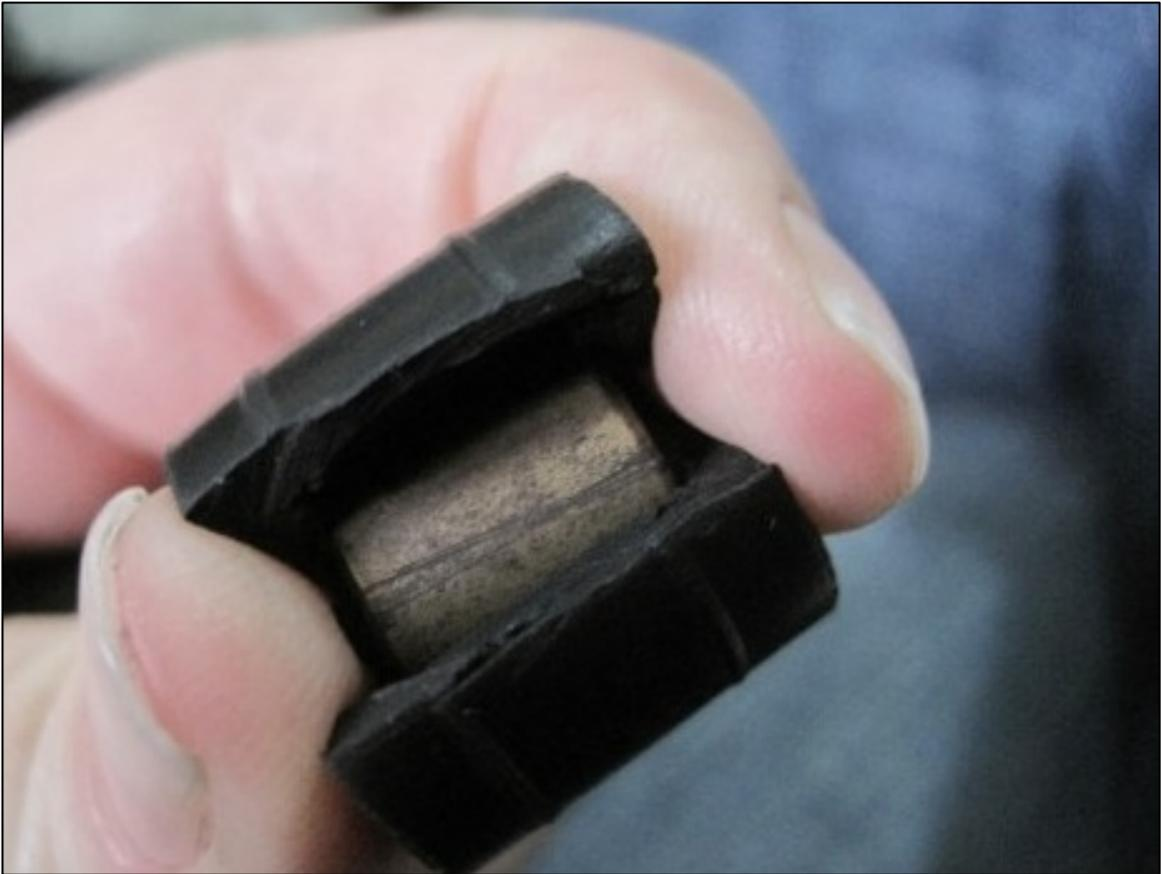
▲ Rubber coated metal bullet showing metal core
