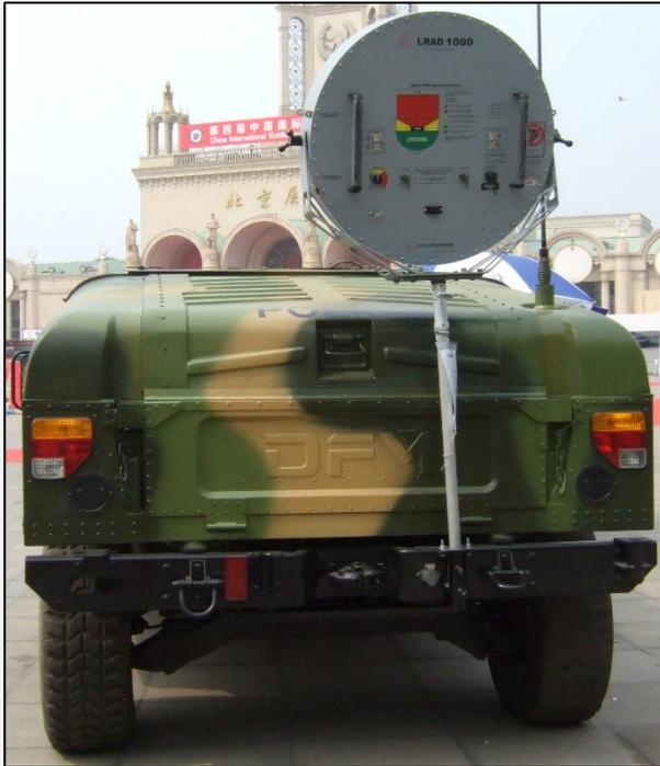
◀ **Vehicle-mounted acoustic hailing device**
