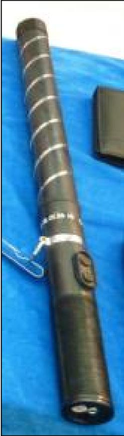
▲ Electric shock baton with metal spiral electrode
